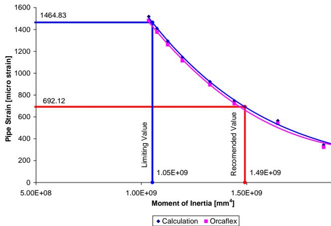
From the strain stiffness graph it is seen that the model test and computer simulation values are very close.
